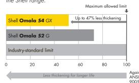
Thickening time (% of limit) (ASTM D2893)
